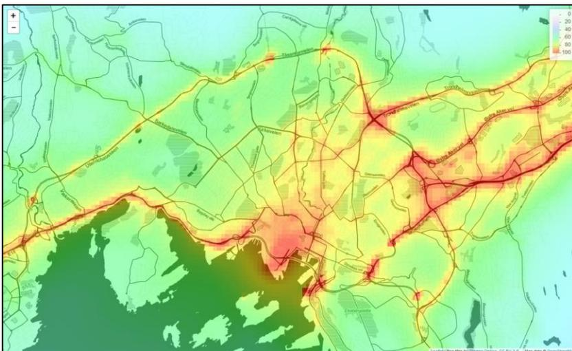
An example of a high-resolution urban air quality map for Oslo, here showing the concentration of nitrogen dioxide (in units of  $\mu\text{g}/\text{m}^3$ ) on a day in January 2016. The map combines the information from 24 AQMesh sensors deployed throughout the city and additional information coming from the EPISODE urban air pollution dispersion model.
